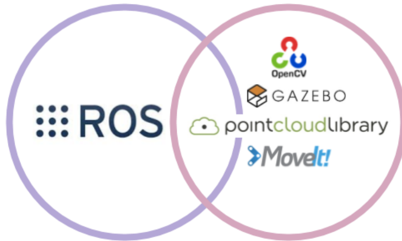
Figure 2.2: ROS includes bindings and integration with many other important open-source software tools.
